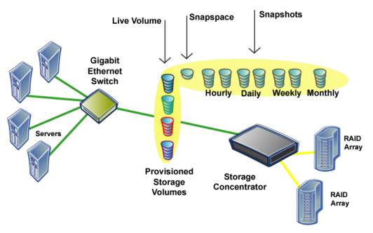
The Storage Concentrator can automatically take Snapshots at predetermined intervals using the Snapshot scheduler. Administrators can configure the system to automatically take Snapshots hourly, daily, weekly and monthly.
